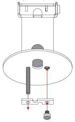
**2** Place in the slot on the fixture.
