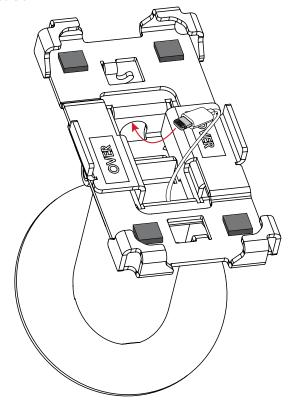
FOR TABLET BRACKETS ONLY: Align the holes on the tablet bracket bar to the holes on the riser. Use the two included screws to secure the bar into place.
