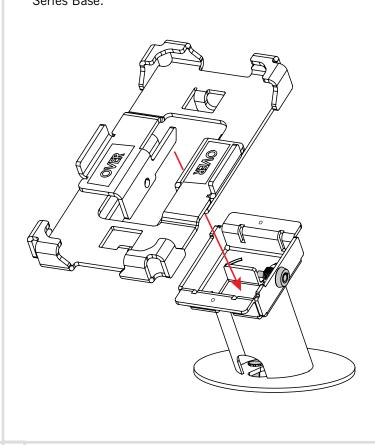
Peel the backing off of the foam and place it onto the device bracket.
