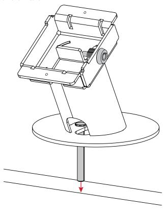
From the underside, slide the circular mounting plate all the way over the post with the gap facing the front of the position.
