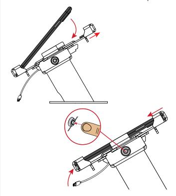
8 Insert the key into the barrel lock and turn clockwise to unlock. Push on the cylinder in the middle of the lock to re-lock.
