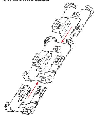
2 Seat the device brackets onto the XD Guardian D Series Base.
