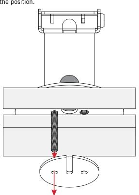
Insert the wing screw into the empty hole on the underside of the riser via the hole in the circular mounting plate. Tighten the wingnuts onto the posts.
