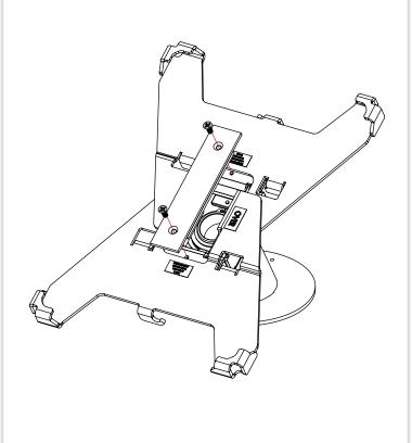
**7** Slide the top half of the device bracket up, and place the product in the bracket. Slide the top half of the device bracket down to snugly fit around the product. Press the barrel lock to lock the brackets into place.
