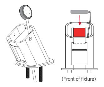
Connect charging cable in correct orientation to watch. The crown and charging cable must be aligned.
