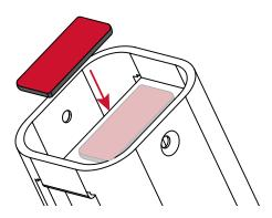
Insert charger into stand. Wires from charger must exit to the right and down into the post. (Facing fixture)
