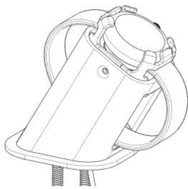
When tightening screws, ensure they do not pinch charger wires as this may damage the charger.
