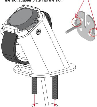
Slide backing plate onto stud(s) on underside of fixture surface and attach wing nuts or screw knob. Tighten until snug.
