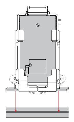
Hold the position steady with one hand. With your other hand use the Double-Sided System Tool to turn the screws to move the mounting tabs into position. Tighten screws to lock position to the fixture.
