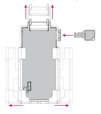
Place the phone on the position, but not over the button. Slide the side brackets in to fit the phone, then slide the phone all the way down over the button.
