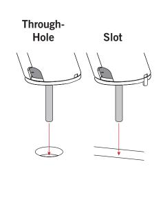
From the underside, slide the mounting plate all the way over the post with the gap facing the front of the position. Tighten the black knob onto the post.
