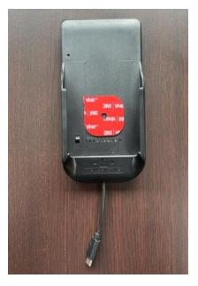
2. Peel off the red adhesive pad film, then take the back cover of the e285 device and align within the payment cradle by hovering over the adhesive pad. Once aligned properly, firmly install the back cover to the adhesive pad.
