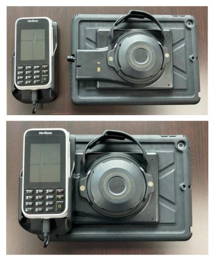
5. To disable the quick release feature of the payment cradle in order to keep the payment device secured, use the red handled tool and turn clockwise via the slot located on the top left corner of the payment accessory.
