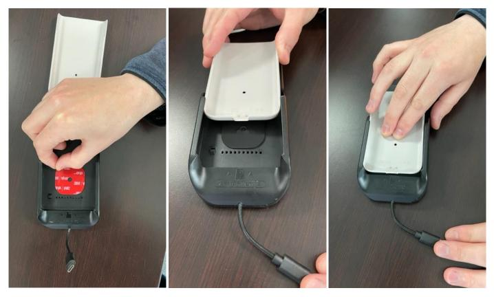
3. Then take the e285 payment device and install by sliding into the payment cradle. Afterwards plug the USB-C Cable into the Verifone e285 payment device.
