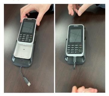
4. Once the Verifone e285 device has been installed, you can now finalize installation by sliding the payment cradle onto the EZ Back utilizing the accessory wing.
