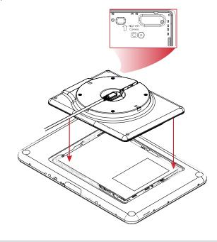
**3** Very carefully secure the SmartBack to the tablet, applying light force to the Hex Key to tighten the 4 corner screws.
