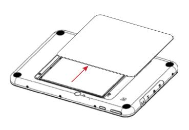
2 Place the VESA SmartBack into the battery opening. Make sure that the arrow on the inside of the SmartBack points to the Tablet Camera.
