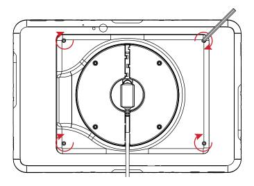
If you have access to a torque screw-driver, Aava recommends setting the driver to 1.23 inch-pounds of torque, or 14 newton centimeters.
