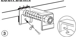
Thread the Screw Cover and Phillips Screw into the PowerBar™ Adapter and tighten with a Phillips Screwdriver. Close Screw Cover Cap when finished.
