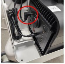
• Confirm the barrel connector from the power supply is plugged into the correct port on the battery:
