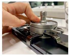
Then, the adapter can be separated from the bracket. Follow normal steps for removing the SpeedBracket (loosen the 2 security screws on the back and slide out the arms).
