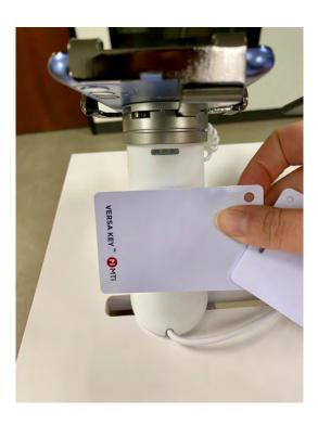
Lift the phone in its bracket out and disconnect the charging cable from the phone. Note that the phone can only be lifted while in portrait orientation.
