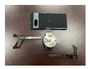
Place the side bracket arms (PS1) on the device, lining up with where they need to fit on the phone.
