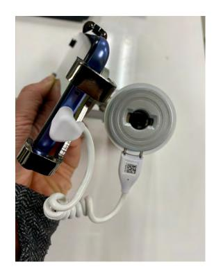
Insert the phone in its bracket, with the adapter attached, into the riser. The adapter stem is keyed to prevent incorrect insertion.
