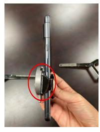
4 Slide in only the bottom bracket arm (PL2) part way, not all the way flush with the device.
