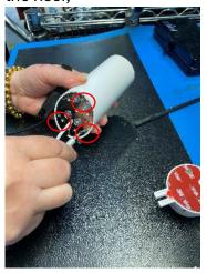
2) Insert crescent end of MTI tool into puck and twist to release the puck from the tether.
