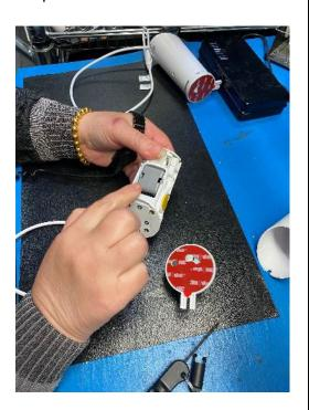
10) Put the riser sleeve back on and tighten the screws you loosened in Step 3.
