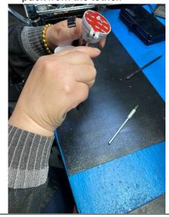
OR use the MTI tool to loosen the 2 screws inside the riser.
