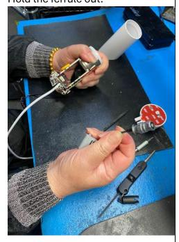
8) Insert the ferrule into the hole inside the riser, then push in the tether assembly.
