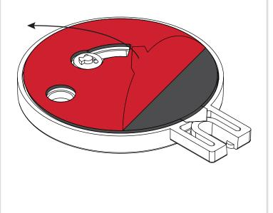
Apply the SpeedPlate<sup>™</sup> to the phone, with the cable retainer towards the charge port of the phone. Use the SpeedPlate cable retainer as alignment reference. Apply firm pressure against the SpeedPlate to the phone for a minimum of 10 seconds.
