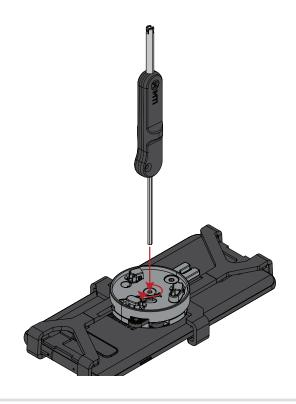
**6** Place pressure on the top/bottom and the sides to try and move arms. This is to find if the arms did not seat correctly.
