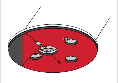
Place Micro position in desired location. Press down on the base plate for 10 seconds for full adhesive contact. Allow 24 hours for full adhesion.
