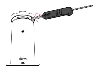
3 With the Freedom Micro® II tool held in the twisted position, rotate the SpeedPlate™ counterclockwise.
