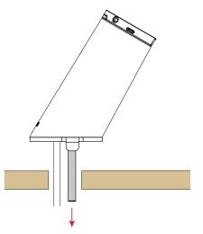
Place the power cable into the slot on the bottom plate, then slide it up over the slot adapter post.
