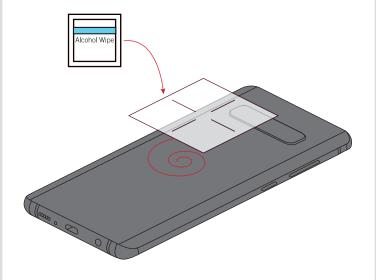
Peel red backing off of the adhesive on the SpeedPlate™.
