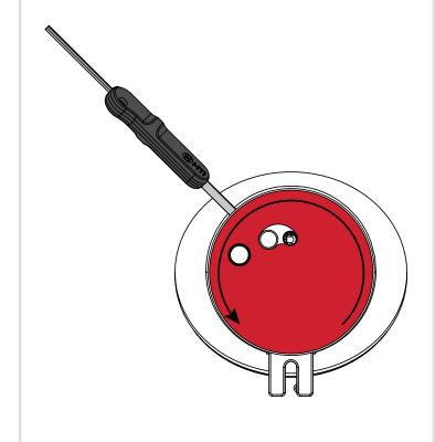
A Remove the SpeedPlate™ from the Freedom Micro® II Puck, then release and remove the Freedom Micro® II tool.
