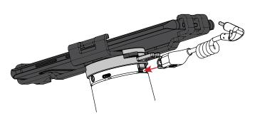
Plug SmartCable into the charge port of the device. LED on back of puck will illuminate solid white when plugged in.
