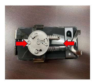
Make sure the bracket arms are not obstructing any needed buttons on the edge of the phone. If further adjustment is needed, repeat above steps until the bracket arms are lined up where they need to be.
