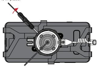
**2** Twist the device and bracket off of the position.
