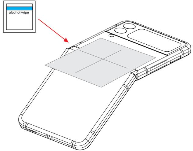
5 Apply phone to hub, aligning the top of SpeedBracket™ hub just below phone hinge line, and centering horizontally. Cable clip on hub should be facing charge port on phone. Apply pressure on hub to ensure VHB adhesion.
