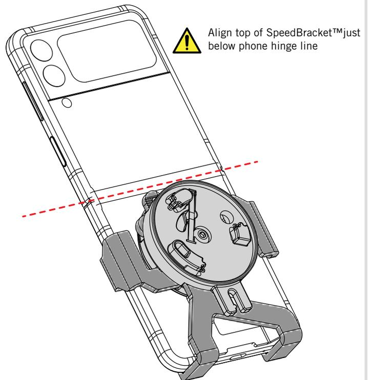
6 Squeeze SpeedBracket™ arms tightly together.
