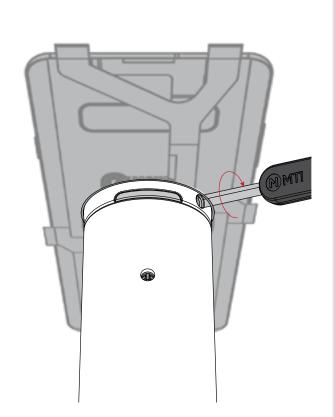
4 Remove the SpeedBracket<sup>™</sup> from the Freedom Micro<sup>®</sup> II Puck, then release and remove the Freedom Micro<sup>®</sup> II tool.
