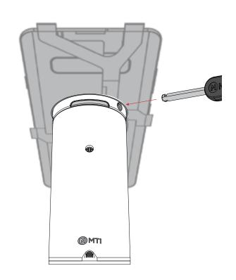
**3** With the Freedom Micro<sup>®</sup> II tool held in the twisted position, rotate the SpeedBracket<sup>™</sup> counterclockwise.
