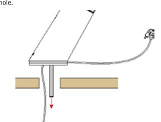
**2** Align bottom plate to slot adapter.
