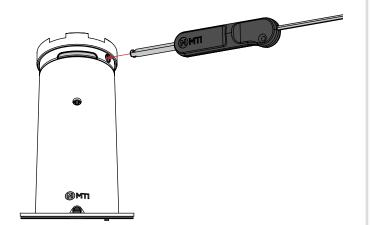
3 With the Freedom Micro® II tool held in the twisted position, rotate the SpeedPlate™ counterclockwise.
