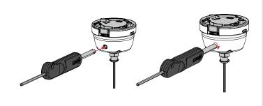
Once the puck is loose, rotate the puck 45 degrees counterclockwise in relation to the tether. Lift the puck off of tether connection.
