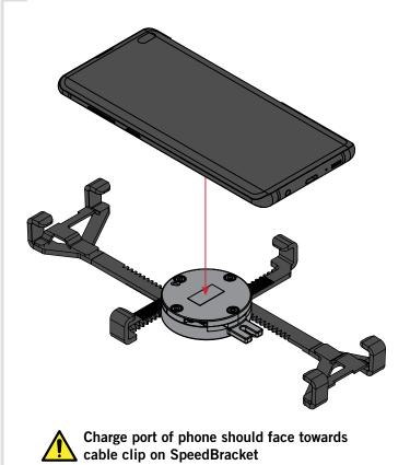
**4** Adjust the universal bracket to fit the device snugly.
