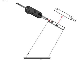
Lift puck out of riser, insert the crescent end of the Freedom Micro II tool into the opening below the charge port on the puck. Twist the Freedom Micro II tool counterclockwise to unlock the puck from the tether.
