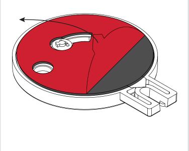
Apply the SpeedPlate™ to the phone, with the cable retainer towards the charge port of the phone. Use the SpeedPlate cable retainer as alignment reference. Apply firm pressure against the SpeedPlate to the phone for a minimum of 10 seconds.
