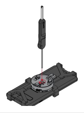
Place pressure on the top/bottom and the sides to try and move arms. This is to find if the arms did not seat correctly.
