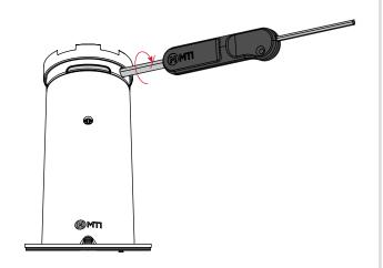
Remove the SpeedPlate<sup>™</sup> from the Freedom Micro<sup>®</sup> II Puck, then release and remove the Freedom Micro<sup>®</sup> II tool.
