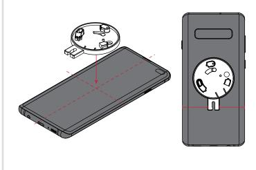
Place the device onto the puck and rotate the device clockwise on the puck until it locks into place.
