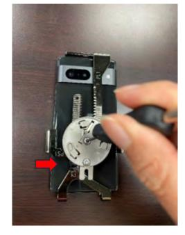
**8** Tighten the 2 security screws on the back.
