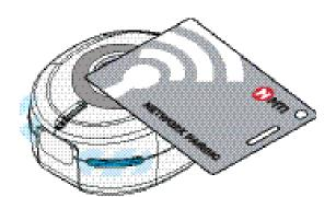
2 Swipe Pairing card to lock. Lock will start slowly beeping confirming it is looking for Connect network. Upon successfully pairing the lock will emit a double beep. Lock will automatically download key whitelist from network.
