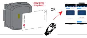
2 Swipe Pairing card to lock. Lock will start slowly beeping confirming it is looking for Versa EX network. Upon successfully pairing the lock will emit a double beep. Lock will automatically download key whitelist from Versa EX.
