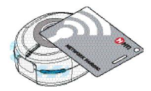
2 Swipe Pairing card to lock. Lock will start slowly beeping confirming it is looking for Versa EX network. Upon successfully pairing the lock will emit a double beep. Lock will automatically download key whitelist from Versa EX.
