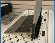
2. Ensure that the ridges on the top of the bracket are positioned to the front. Next, center the laptop between the legs.
