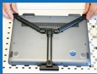
4. Press the two corner legs into the crease of the laptop, so they are nice and snug against the device. Tighten the legs.
