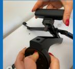
2. Remove wingnuts. Align the studs with the holes in the fixture. Tighten the wingnuts on all sides.
