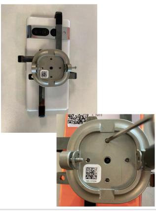
8 Install the puck and tighten the 2 security screws on the back using the MTI tool.
