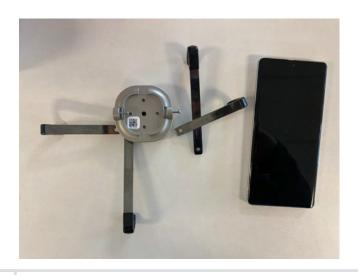
4 Slide in only the bottom bracket arm part way, not all the way flush with the device.
