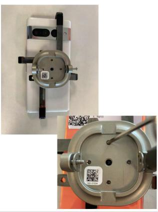
Make sure the bracket arms are not obstructing any needed buttons on the edge of the phone. If further adjustment is needed, repeat above steps until the bracket arms are lined up where they need to be.
