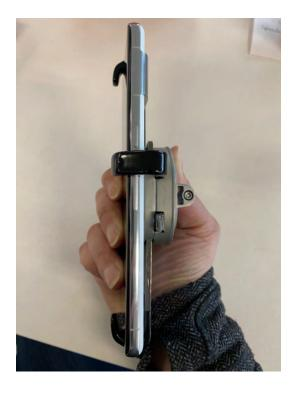
Slide both arms inwards and fit all bracket arms snugly around the device. Tighten the 4 screws using the MTI tool
