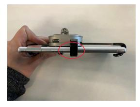
1 Using the Freedom Micro tool, loosen the 4 security screws on the back of the medallion to loosen the bracket arms.
