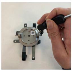
Place the side bracket arms on the device, lining up with where they need to fit on the phone. Ensure the medallion is in the upright orientation; the QR code label should be upright.
