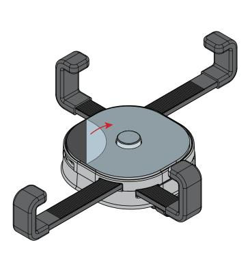
Place device in the bracket and press down for NanoStick to hold in place.
