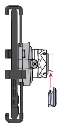
If using the retrofit position bracket, dock the puck, and tighten the 2 captive security fasteners to either side of the puck through bracket stirrup.
