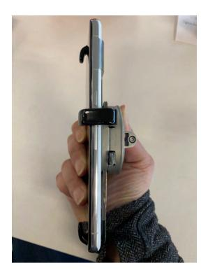
4 Tighten the security screws on the back using the MTI tool.
