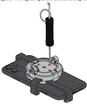
Double-check that arm screws are fully tightened! Also, check arms monthly to ensure they are tight. Arms may loosen over time with use. Insert puck without VHB and tighten the 2 captive security fasteners to either side of the puck. If using retrofit lockdown bracket, insert puck, then proceed to steps 7 and 8.
