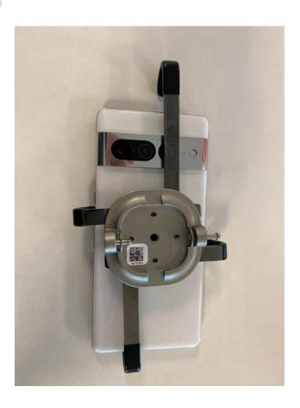
6 Slide both arms inwards and fit all bracket arms snugly around the device. Tighten the 4 screws using the MTI tool.
