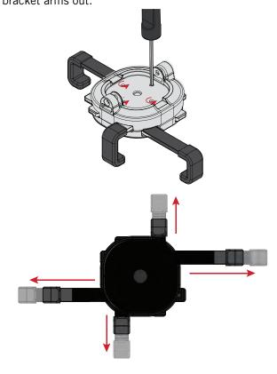
For new brackets, peel clear film off of NanoGrip. If reusing bracket, nano-grip can be cleaned with water and a soft cloth.
