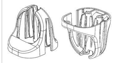
2 Slide watch and charger into watch enclosure top with watch bands in slots
