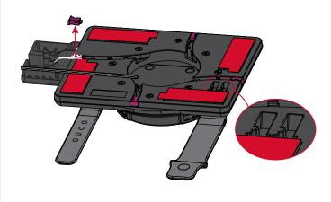
Route the cable(s) through the cable channel, starting counter-clockwise in the center cable channel.
