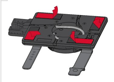
**5** Place the EZ Back on the back of the tablet. Then, plug in the power connector while pushing the extra cable into the EZ back.
