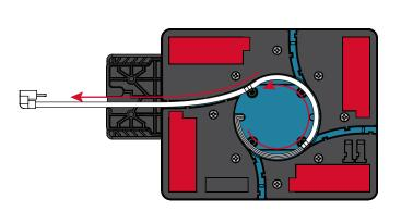
**4** Peel the red film off of the adhesive tape on the EZ Back.
