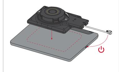
For full adhesion, use a rubber band to hold the EZ Back in place for 24 hours before using.
