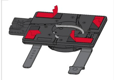
Place the EZ Back on the back of the tablet. Then, plug in the power connector while pushing the extra cable into the EZ back.
