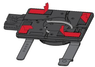
Place the EZ Back™ into the hole on the back of the TPU case with the power cable on the same side as the power port of the tablet.
