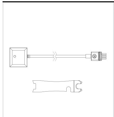
Insert tool into cable housing and push firmly. This will allow cover to open.
