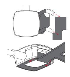
Remove backing of adhesive on the FlexSensor in preparation for attaching to back of watch.
