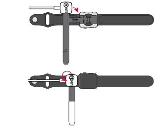
12 Wrap loop around and insert end of loop through anchor housing. Tighten FlexSensor, remove backing of adhesive and adhere to underside of sensor. There may be some excess material at the end which may be trimmed off. Remove Intellikey from Alarm Module to arm system.
