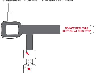
10 Firmly press FlexSensor adhesive side down on back of watch as shown.
