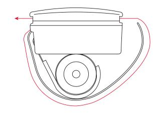
Tighten FlexSensor, then peel VHB and the end of the FlexSensor and adhere to underside of anchor.
