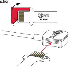
Align cable to the stylus pen with the sensor on the curved part of the pen, leaving the flat side available to mount to the iPad. Remove VHB backing from FlexSensor and place on the stylus pen.
