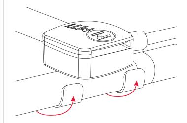
Feed FlexSensor through the top of the FlexTech cable and continue to wrap around stylus pen.
