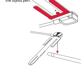
3 Wrap adhesive FlexSensor around the stylus pen.
