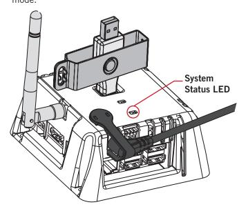
2 Cycle the power to the Network Extender by unplugging and re-plugging the connection at the POE power adapter 3 times. Upon re-connecting the 3rd time, the Network Extender LED will flash blue.
