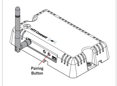
When the Network Extender attaches to the mesh network, the blue flashing LED will become solid Green. If the Network Extender does not connect to a mesh network within 90 seconds, it will exit pairing mode and will return to its previous state.
