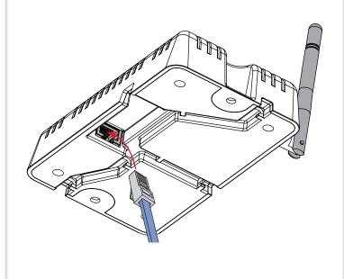
Mount the extender using the 3.5 mm x 16 mm screws (or longer if needed) for the mounting surface (not included).
