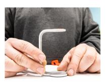
Place stand onto fixture. Apply pressure to VHB for 10 seconds. Apply pressure to the edges and center of stand to ensure full adhesion. The angled top surface should be oriented towards the front of the fixture.
