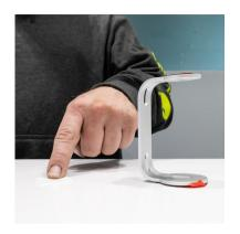
Clean fixture surface with alcohol wipe. Allow to dry thoroughly.
